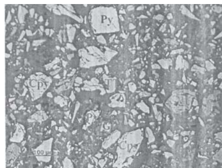
Fig. 2. Sample CC1 00, reflected light: Cpy-chalcopyrite, Py-pyrite, Bl-blenda, Gl-galena, a-sulfates tire, TT-tenantite-tetraedrit
